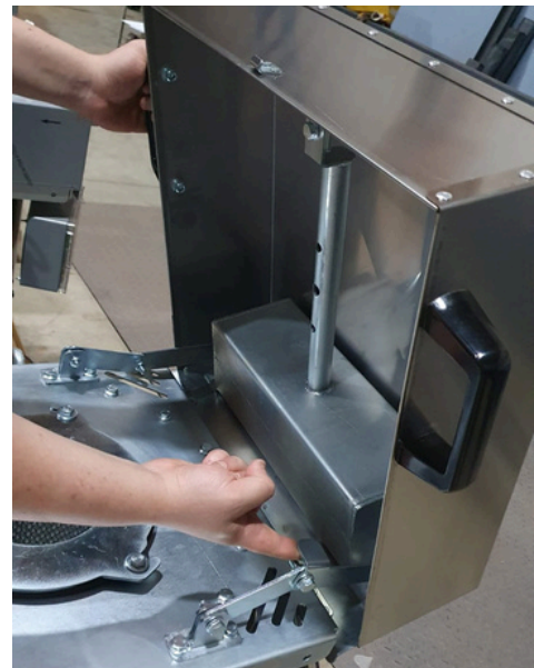
4 - After changing/cleaning the cartridge, pull the cover from left handle and push the right lock up as shown.
