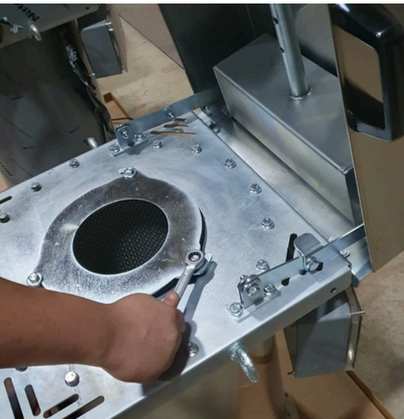
3 - Release the the bolts with an 13 spanner and take the cartridge off.
